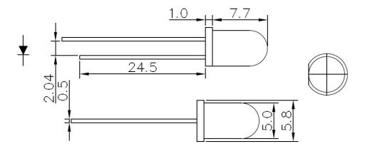
Note: Besides to the specified outside, all units in mm, a tolerance of  $\pm\,0.20$ mm
